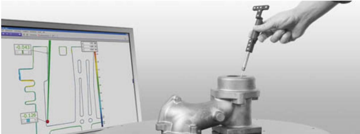
Our Inspection technologies enable the rapid acquisition of the most complex of forms and provide immediate feedback as to their integrity.
