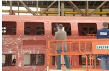
GOM's portable metrology systems support production controls and inspection of repairs and maintenance performed on railroad car bodies. They analyse inspection criteria that include body-in-white levelling to ground and wheel set, wall perpendicularity, and dimensions and distortions for door and window openings. GOM's TRITOP<sup>CMM</sup> system handles:
