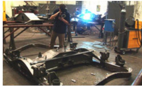
TRITOP<sup>CMM</sup> system, one person can typically inspect a bogie and create a measuring report within forty minutes. An automatic evaluation routine aligns the measured data with the nominal data, calculates any deviations, and prepares and prints the final measuring report.
