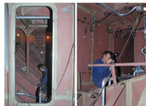
However, GOM systems can be used to create a 3D design of the compartment geometry within a few hours. The 3D data is then used as direct input for CAD systems, making units easy to design, build and integrate smoothly into existing compartment structures.
